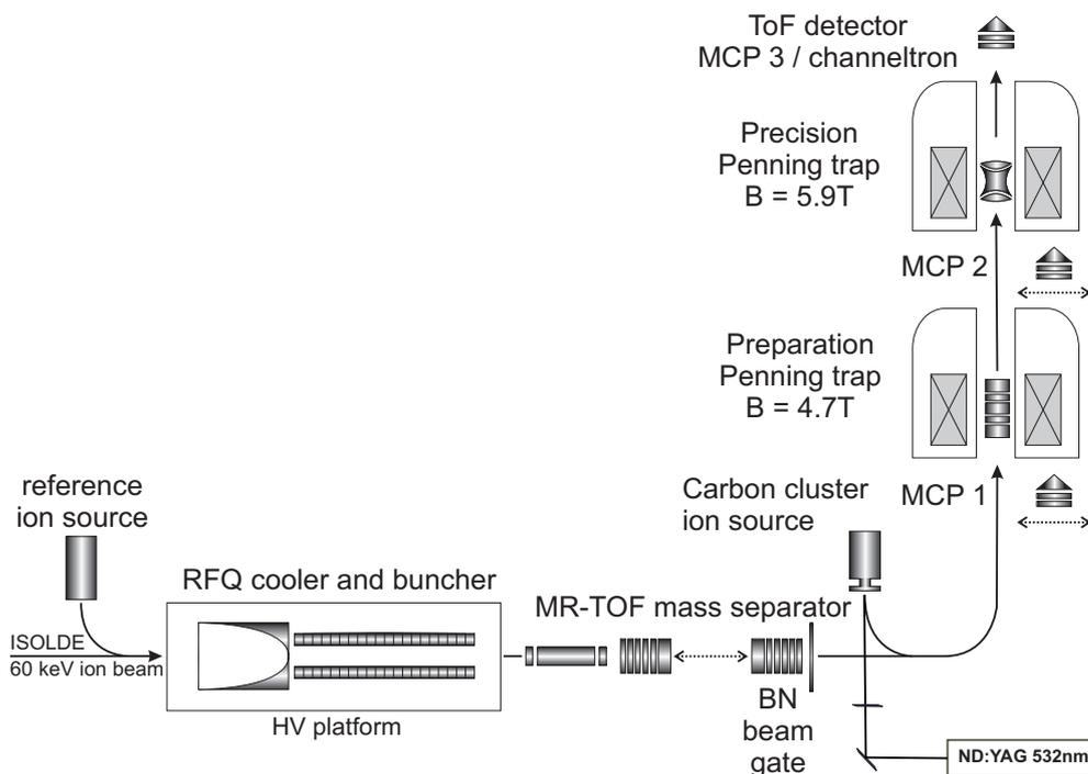
Figure 3: Schematic view of ISOLTRAP. For details see text.
