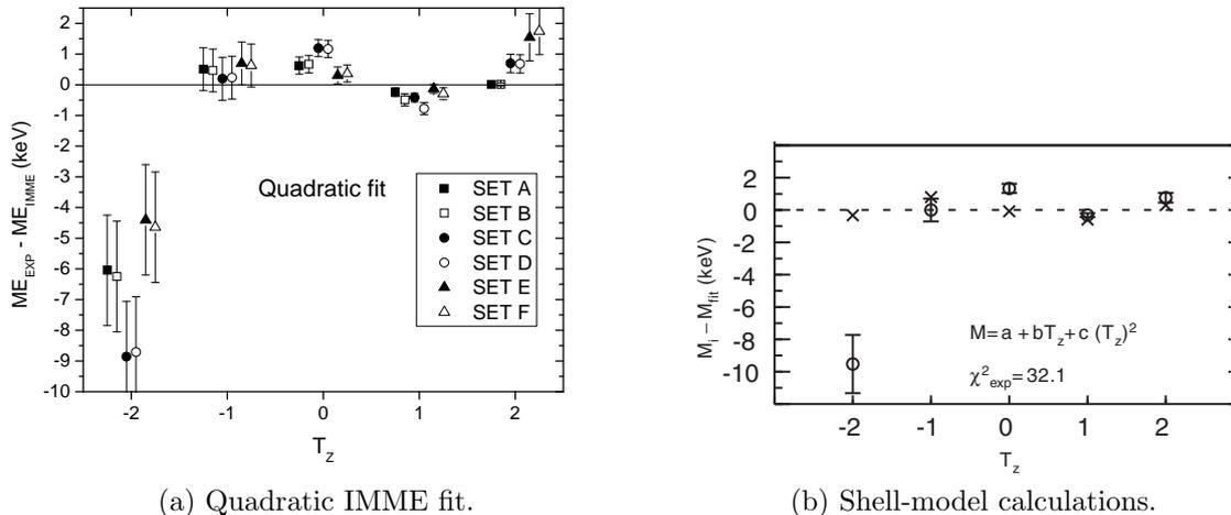
Figure 2: (a) Differences of the experimental values to the error-weighted quadratic fits of the mass-excess values in the  $T = 2$  quintet at  $A = 32$  from different measurements, cp. Tab. 1. The error bars represent only the uncertainties of the experimental mass-excess values. (b) Accuracy of the IMME with three terms (circles) and corresponding theoretical calculations with the USDB interaction (crosses). Taken from [7].
