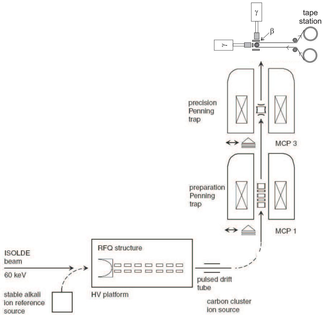
Figure 5: The triple trap mass spectrometer ISOLTRAP along with the proposed decay spectroscopy setup.
