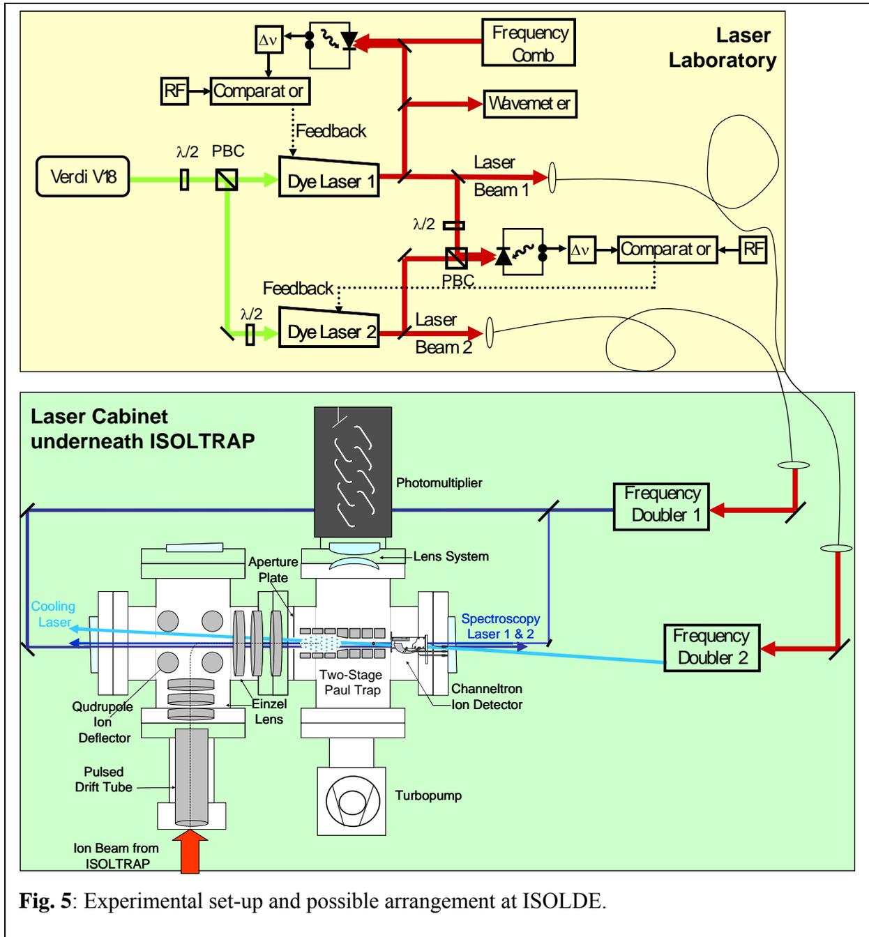
**Fig. 5:** Experimental set-up and possible arrangement at ISOLDE.
