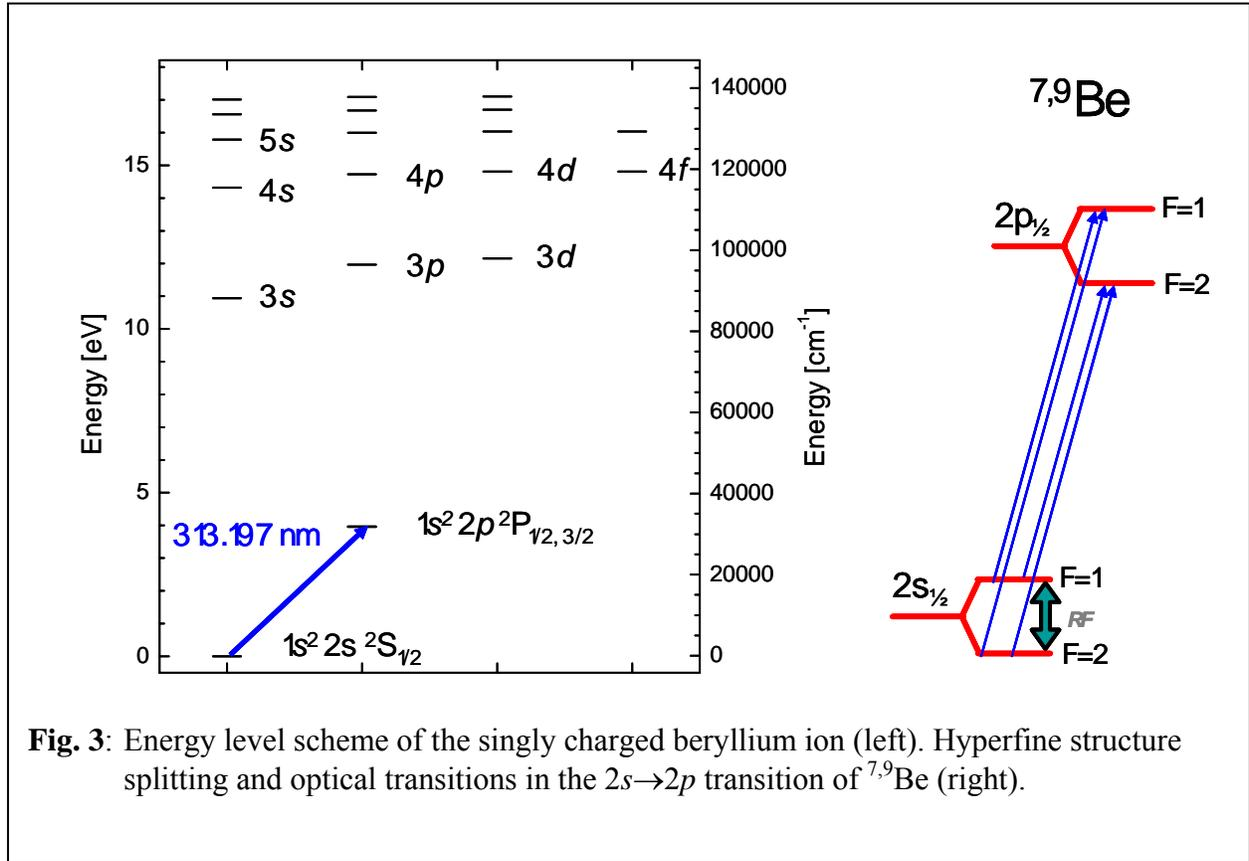
**Fig. 3:** Energy level scheme of the singly charged beryllium ion (left). Hyperfine structure splitting and optical transitions in the  $2s \rightarrow 2p$  transition of  $^{7,9}\text{Be}$  (right).
