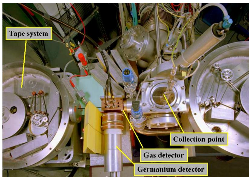
Figure 3: *Experimental setup as used in the GSI experiment to measure the half-life of  $^{62}\text{Ga}$  with high precision [9].*
