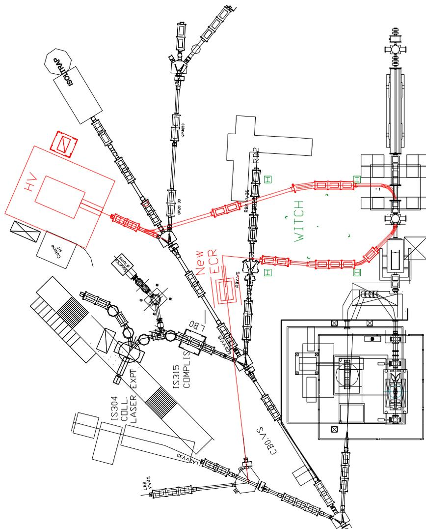
Figure 4: Beamlines for extraction and injection of the low energy high charge state ion beam of the REX facility suggested in this study (courtesy of H. Haas).
