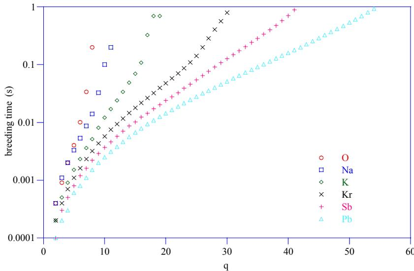
Figure 3: Breeding times as a function of the charge state for a current density of  $200 \text{ A/cm}^2$  (courtesy of F. Wenander [Wen01]).
