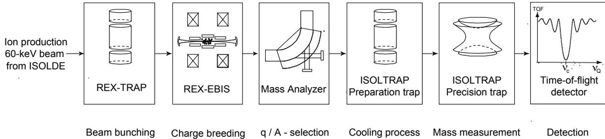
Figure 1: Schematic layout of the electron beam ion source (REX-EBIS) and the Penning trap system (ISOLTRAP).
