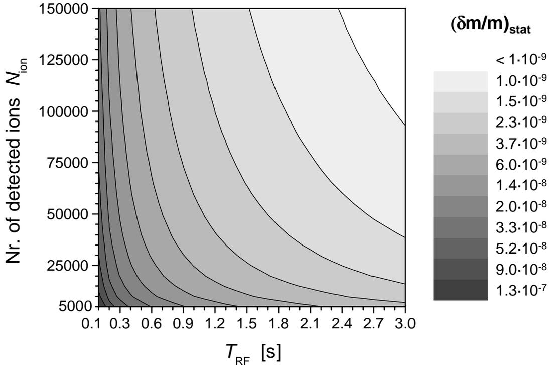
Figure 5: The statistical uncertainty  $(\delta m/m)_{\text{stat}}$  as a function of the observation time  $T_{\text{RF}}$  and the number of detected ions  $N_{\text{ion}}$  for an ion with mass number  $A = 100$  in a magnetic field of  $B = 6$  T.
