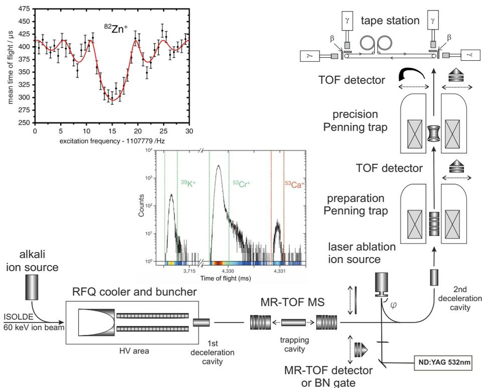
Figure 1: Schematic view of the ISOLTRAP setup. The inset on the left shows a time-of-flight ion-cyclotron resonance of  $^{82}\text{Zn}^+$  (TOF detector above precision Penning trap), the inset on the right shows a time-of-flight spectrum of  $A = 53$  (MR-TOF detector). For details, see text.
